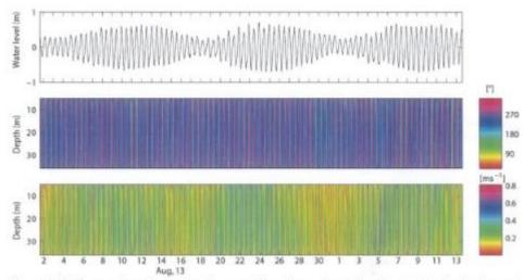
Figure 3-4: Time series of water level, current direction and speed at Oyster Bay during August and September 2013.
