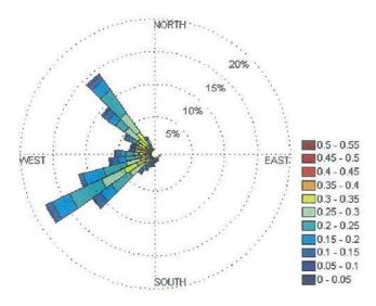
Figure 3-7: Current roses showing percentage distribution of speeds and direction at 20 m in the water column.
