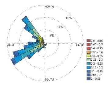
Figure 3-6: Current roses showing percentage distribution of speeds and direction at 12 m in the water column.
