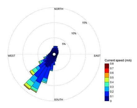
Figure 3-2: Current rose showing current directions and magnitudes for all bins at Blowhole Point North.
