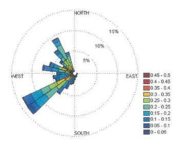
Figure 3-9: Current roses showing percentage distribution of speeds and direction at 34 m in the water column.
