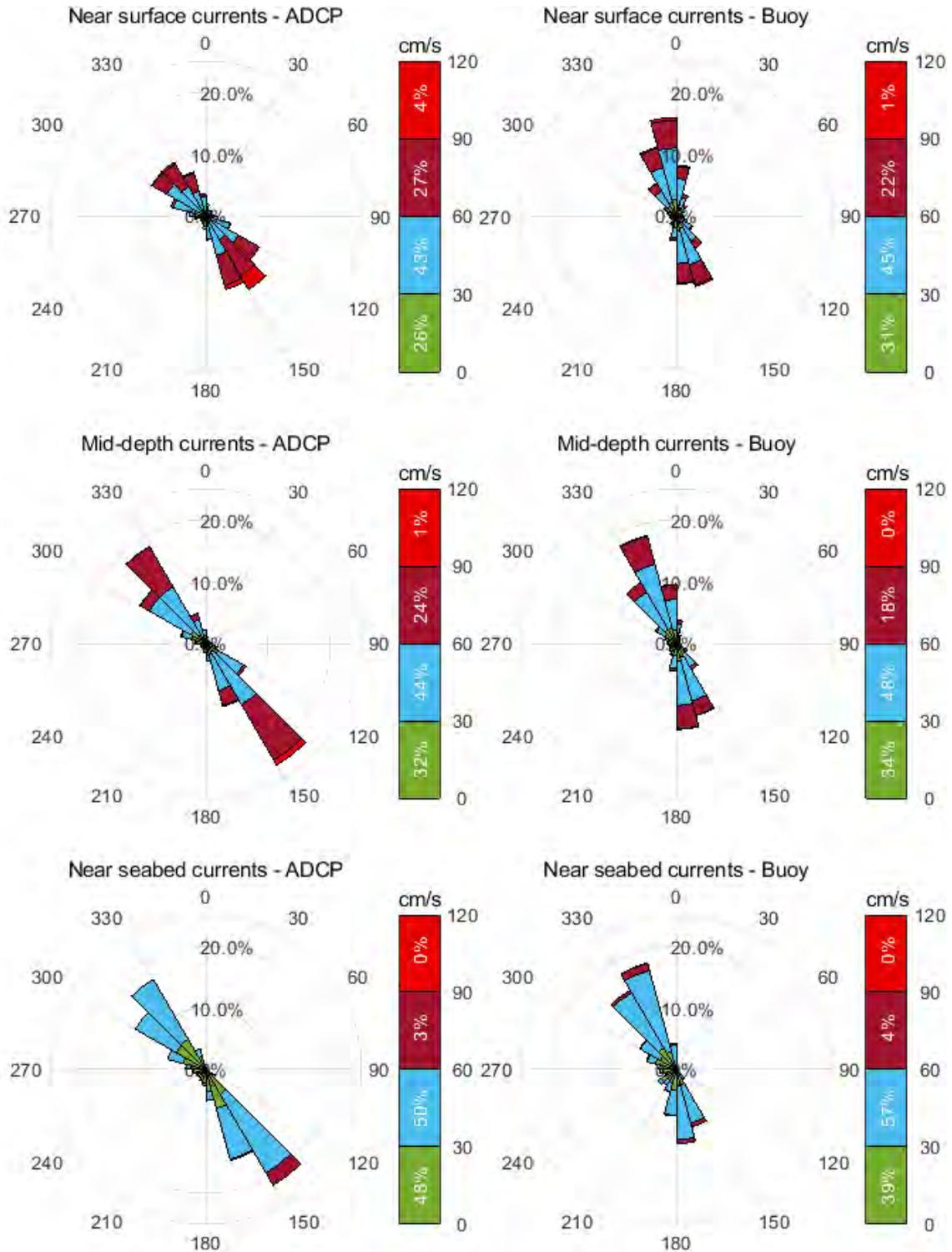
Figure A8.1. Measured current data from the upwards facing ADCP (left) and downward facing ADCP (right) at near-surface, mid-depth and near-seafloor elevations. The directions are in the 'going to' sense; that is, currents at 90 degrees in the rose plot would be travelling from west to east. The white numbers within the colour bars give the percentage of time that current velocities are within that range. For example, mid-depth current speeds exceed 90 cm/s 1% of the time.
