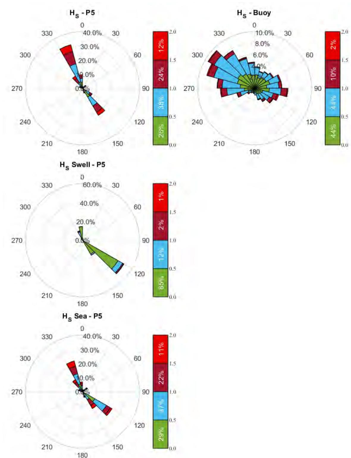
Figure 10. Comparison of measured and modelled wave heights for ‘sea’ and ‘swell’ components at site P5. The directions are in the ‘coming from’ sense; that is, waves at 90 degrees in the rose plot would be travelling from east to west.
