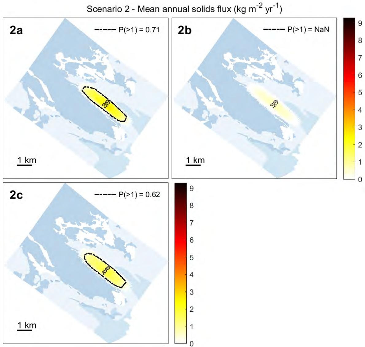
Figure A10.3. Scenario 2 depositional model outputs: different block layouts and different pen size and feed throughputs. The dashed line indicates the boundary of the area where solids flux is  $> 1 \text{ kg/m}^2/\text{yr}$ .  $P$  = the probability of encountering solids flux of  $> 1 \text{ kg/m}^2/\text{yr}$  within that area. The background delineates the epifaunal strata described in Section 2.5.2. Dark areas contain biogenic habitat.
