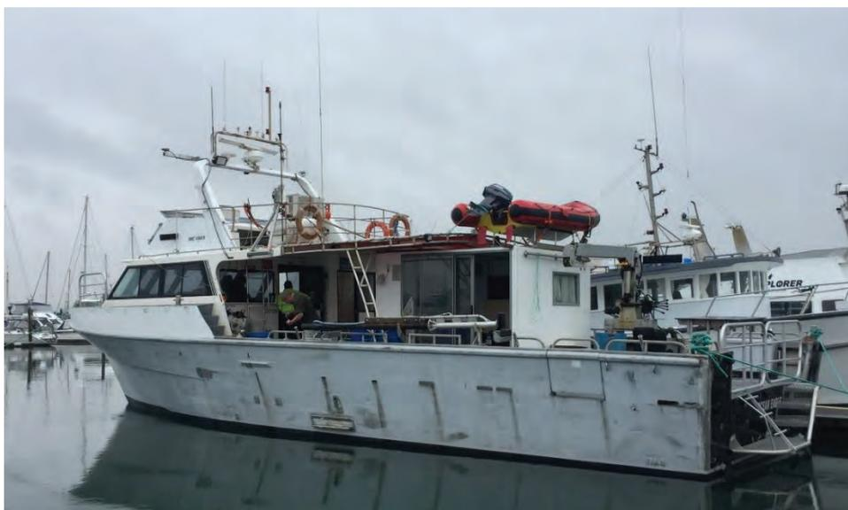
**Figure 2: Ocean Eagle Fitted with MBES Pole**
