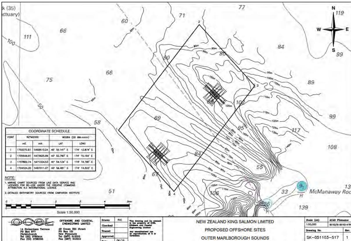
Figure 4.3: OCEL drawing of proposed site<sup>9</sup> showing water depth, shoals and indicative farms and moorings
