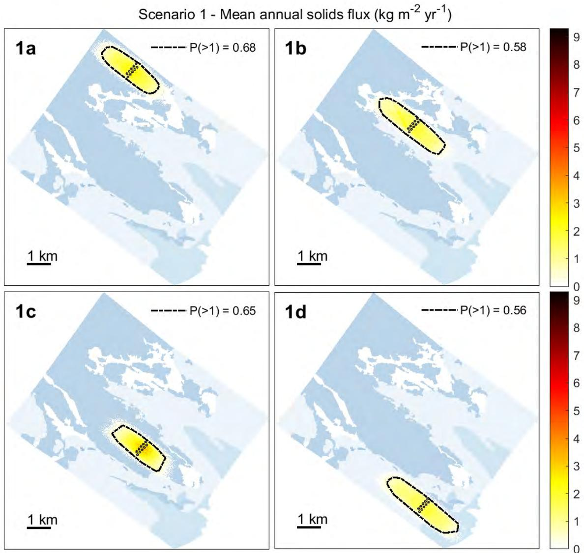
Figure A10.2. Scenario 1 depositional model outputs; multiple locations across the area. The dashed line indicates the boundary of the area where solids flux is  $> 1 \text{ kg/m}^2/\text{yr}$ .  $P$  = the probability of encountering solids flux of  $> 1 \text{ kg/m}^2/\text{yr}$  within that area. The background delineates the epifaunal strata described in Section 2.5.2. Dark areas contain biogenic habitat.
