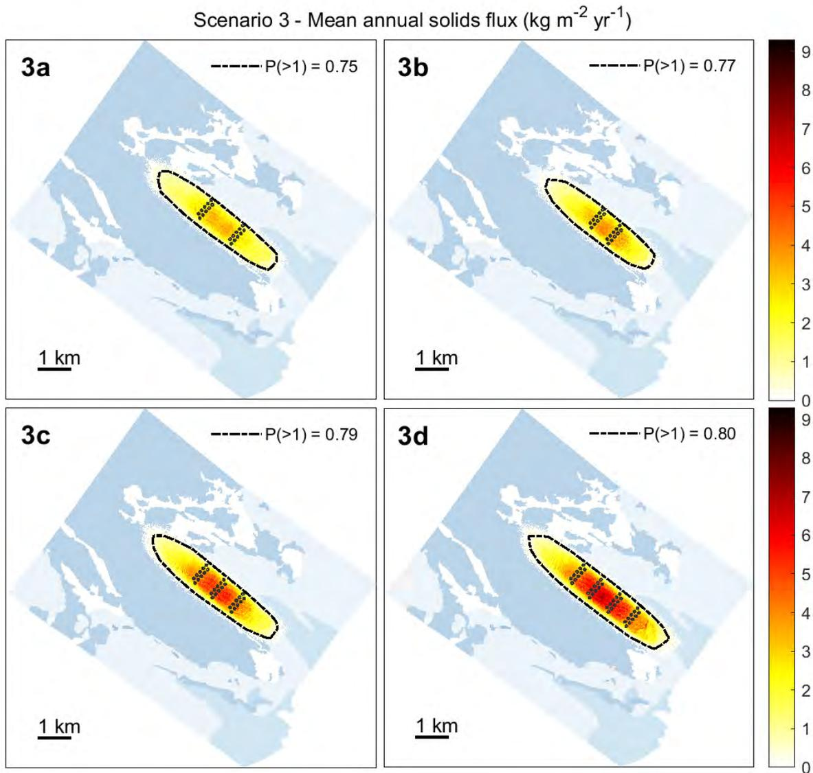
Figure A10.4. Scenario 3 depositional model outputs; same block layouts but increasing footprint overlap. The dashed line indicates the boundary of the area where solids flux is  $> 1 \text{ kg/m}^2/\text{yr}$ .  $P$  = the probability of encountering solids flux of  $> 1 \text{ kg/m}^2/\text{yr}$  within that area. The background delineates the epifaunal strata described in Section 2.5.2. Dark areas contain biogenic habitat.
