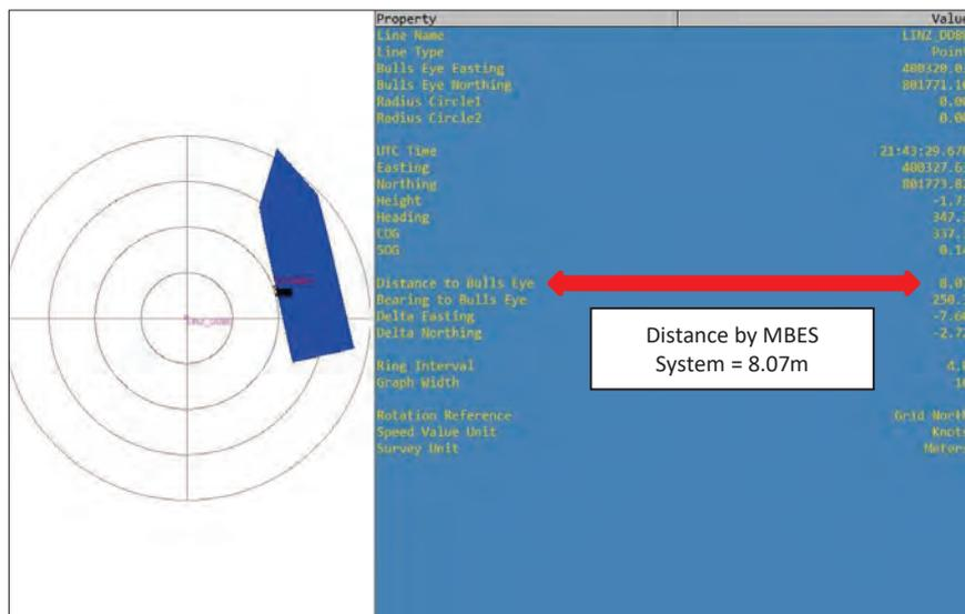
Figure 4: Positioning Check at Queens Wharf Mark DD8U
