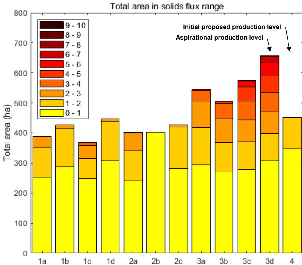
Figure A10.1. Summary of the total area affected by differing amounts of depositional flux (scale shows kg solids/m²/yr) for each of the scenarios modelled in Table A10.1.
