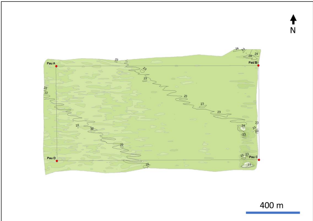
Figure 7: Seafloor hardness and depth contours from the initial survey. The green and paler green colour in the image represents soft sediment.
