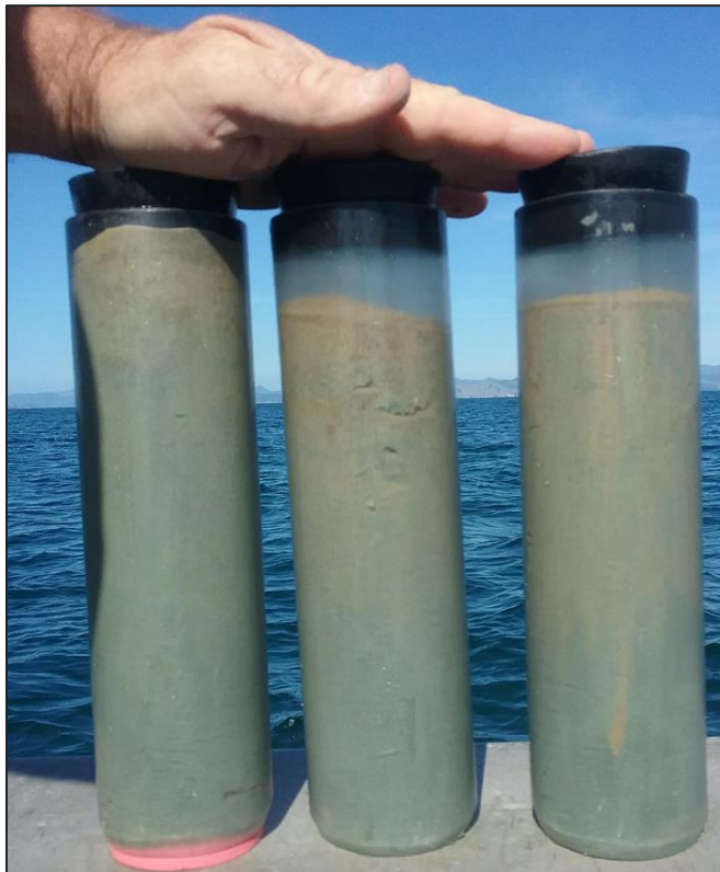
Figure 14: Sediment cores from the initial survey sampled via SCUBA at the dive site
