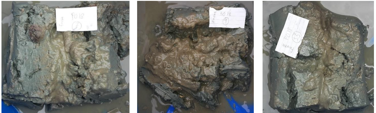
Figure 13: Ponar grab contents from the expanded farm survey at stations 7, 9 and 15 showing the characteristic muddy sediments of the grab samples.
