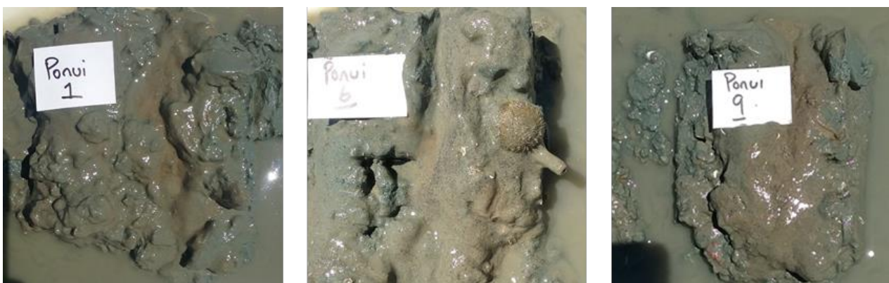
Figure 12: Ponar grab contents from the initial survey at stations Sed1, Sed6 and Sed9 showing the characteristic muddy sediments of the grab samples.
