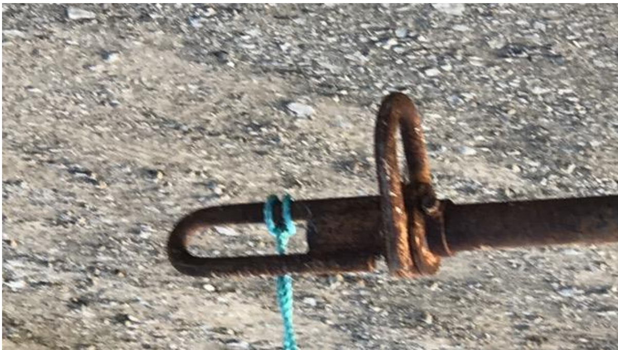
Figure 2c: Eye of the screw anchor, which will be level with the seabed but will not be visible due to the soft mud substrate at the site
