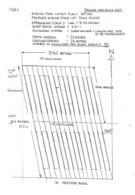
MARINE FARM LAYOUT PLAN : SIDE VIEW. PROPOSES MARINE FARM " DEF PONUL ISLAND. APPROXIMATE SLALE : I MIN = 2:5 METRES. WARP RATIO : 2.5 -1 SCREW ANCHOR - LENGTH AND HELIX SIZE TO BE DETERMINED ANCHODING SYSTEM AVERAGE DEPTH 23 METRES,
