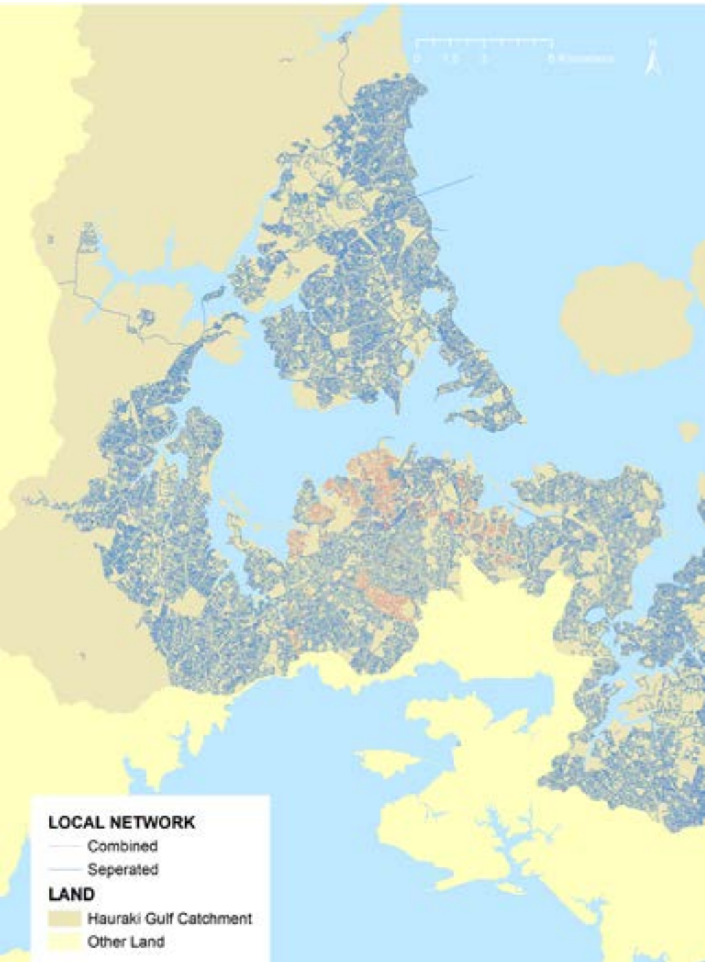
Figure 5.1: Central Auckland areas serviced by a combined wastewater and stormwater pipe network (i.e. both services are included in the same pipe (red)), and areas with separate wastewater pipes (blue).
