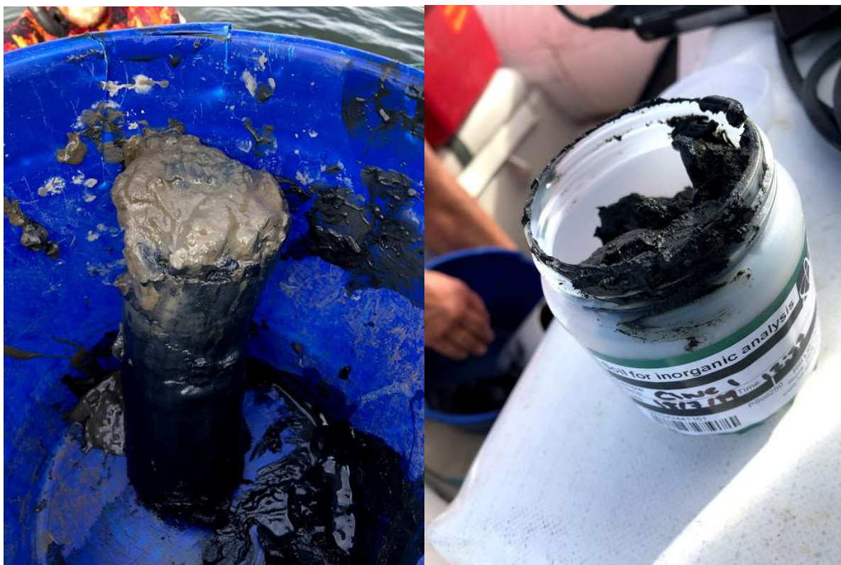
Figure 2.2. A sediment core (left) and sample jar (right). Note, the ~5 mm of surficial sediment above the anoxic material.
