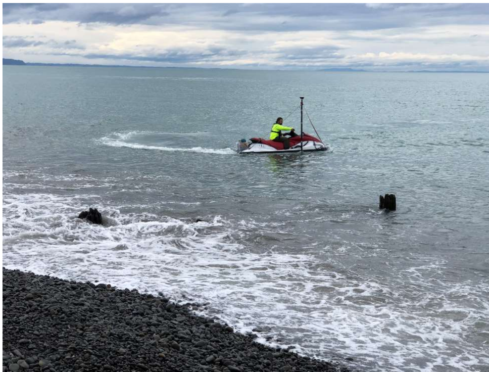
Figure 4.1. Bathymetry surveying on the open coast side of the Clive River entrance.
