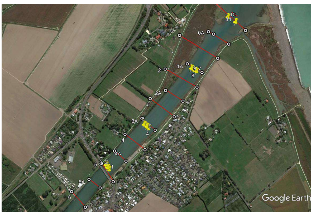
Figure 2.1. The 11 sediment and probe sampling sites are indicated by the yellow markers (the coordinates are presented in Table 2.1), and the digitised transects for dredging volume calculations are shown by the red lines.
