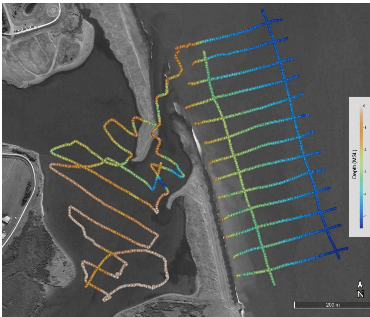
Figure 4.2: Survey data points adjusted to Napier Vertical Datum 2000 overlain on a satellite image from 22 nd May 2019 (Google Earth)
