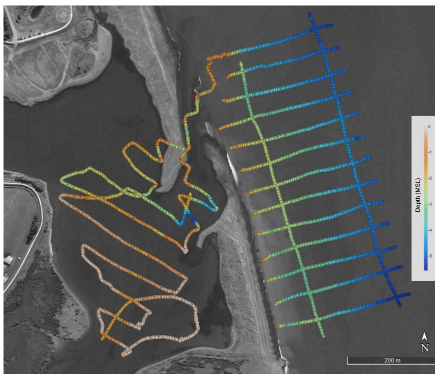
Figure 2.2. Survey data points adjusted to Napier Vertical Datum 2000 overlaid on a satellite image from 22 nd May 2019 (Google Earth). Note, the river entrance was located north of this image on 23 rd August 2019.
