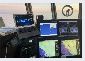
Nelson company Advanced Conservation Solutions (ACS) has created 'DeepSet', a camera with machine learning algorithms to identify in real time fish species entering a trawl net. The DeepSet system has been in development for three years with support from Callaghan Innovation. ACS' DeepSet is currently operating as a prototype in Aotearoa New Zealand waters.
